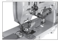
Suit for trimming and taping simultaneous for bedding, cover, cushion and carpet, etc. Trimming can be made in front of needle.
