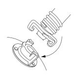
7. Place steam nozzle into hook on top of pole set. Remove protective cotton cover/bag from nozzle. Always return hose to this position when not in use.
