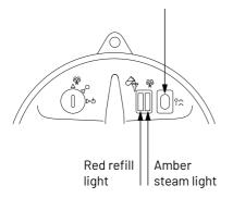
Turn pointer on control knob to steam position, amber steam light will illuminate.
